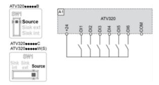
Switch SW1 set to "Source" position and use of an external power supply for the DIs.
