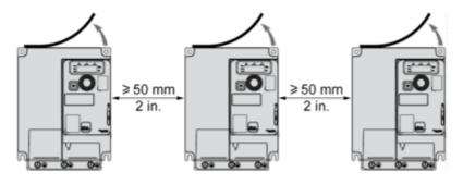
For Operation at Ambient Temperature Above 50 °C (122 °F)
